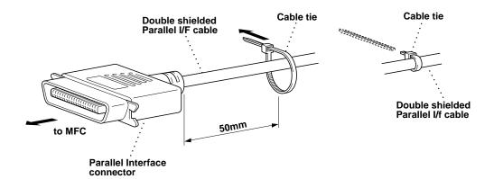
Attach the Cable tie 50mm or less from Parallel Interface connector.
